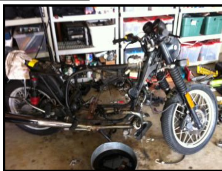
The sad, fascinating deconstruction of a R75/6 with a seized driveshaft. Great experience seeing the entire bike being disassembled.
